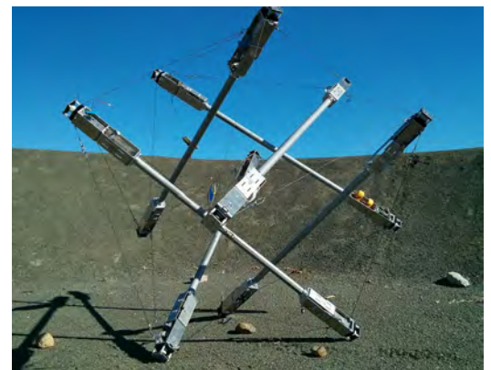
NASA SUPERball Tensegrity Lander Prototype
